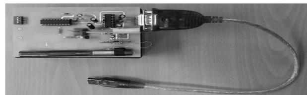
**Figure 3. Evaluation module of MSF receiver.**
