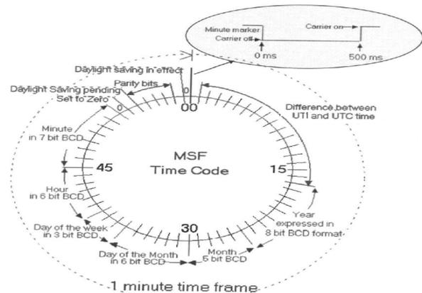
**Figure 2. MSF time and date code signal format, 00-59 seconds, source [15].**
