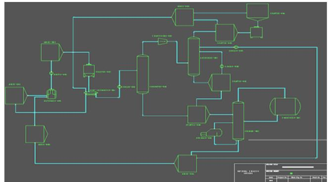
Fig. 7. PFD for the vinyl acetate process of Luyben [12]
